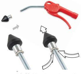
Air Boy® Push-in nozzles are easily mounted by pressing it on the tip of the blow pipe. Remove by pressing the plastic collar forward and push the nozzle off.
