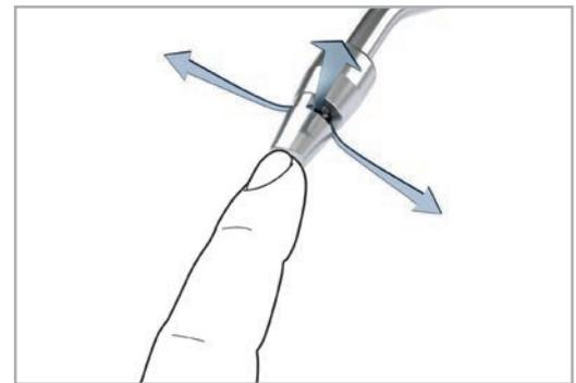
Air Boy® Turbo increases airflow using the ByPass venturi nozzle. It has an unblockable nozzle that lets the air flow through the sides if the tip is blocked.
