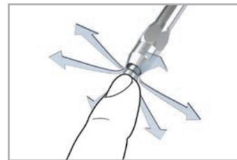
Silent Air Boy® has either an unblockable nozzle that lets the air flow through the sides as illustrated, or a pressure stop, that stops the airflow.
