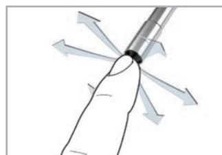
Super Silent Air Boy® has an unblockable nozzle that lets the air flow through the sides if the tip is blocked.
